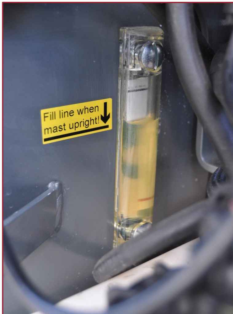
Figure 14 - Oil Tank Gauge
