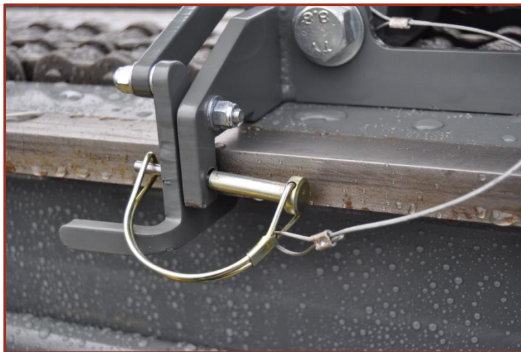
Figure 10 - Kelly bar jack locked onto the mast
