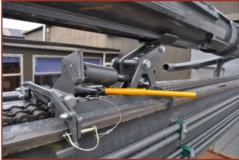
Figure 11 - Kelly bar jack being raised
