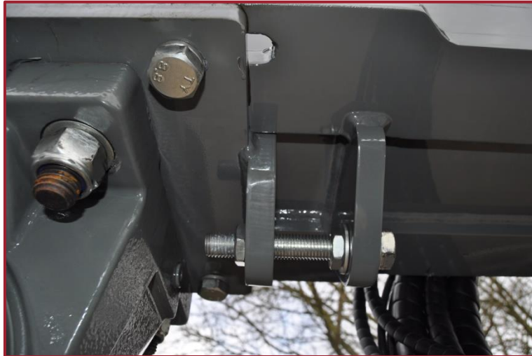
Figure 20 – Chain Drive Adjustment Set Bolt
