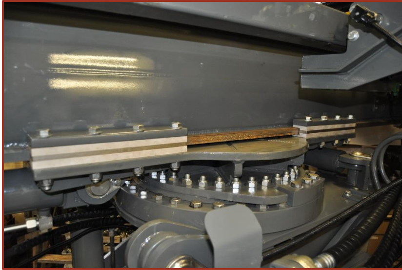
Figure 16 - Mast Wear Pads and Locking Bolts
