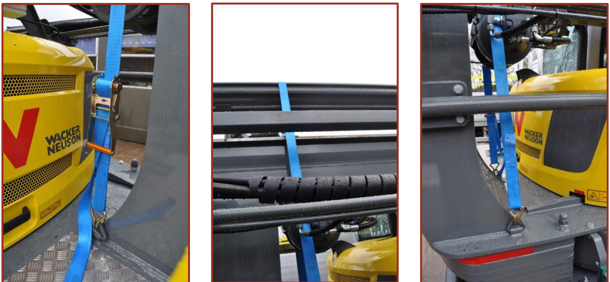
Figure 13 - Kelly bar ratcheted for transport
