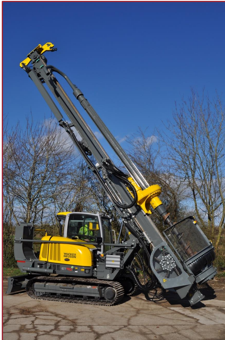
Figure 3 - Standing the Mast Upright
