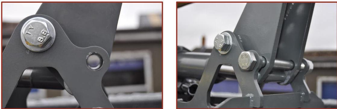
Figure 12 - Kelly bar jack retaining bolt holes and bolt
